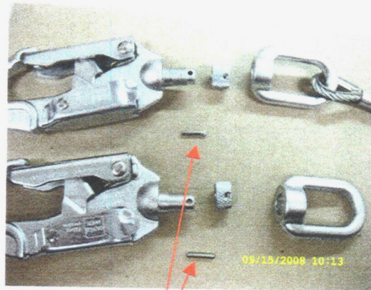
Hook Needs Replacement (loose or missing pin)
