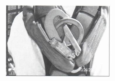
The identified reason for the inadvertent disconnection is the combination of a particular style locking snaphook (9502573) together with twin lanyard legs sewn directly to the eye of the snaphook. Although there have been no reported falls or injuries associated with the use of this configuration lanyard, CS is committed to the safety of every worker at height using our products and we are determined to resolve any potential for inadvertent disconnection to occur for the reason described above.
