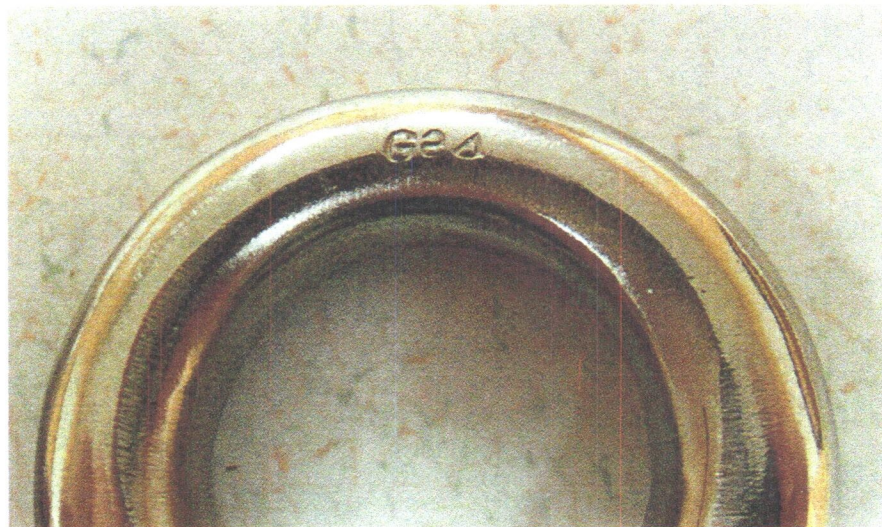
Picture # 2 Reverse side of BAD shackle with "G24" heat code
