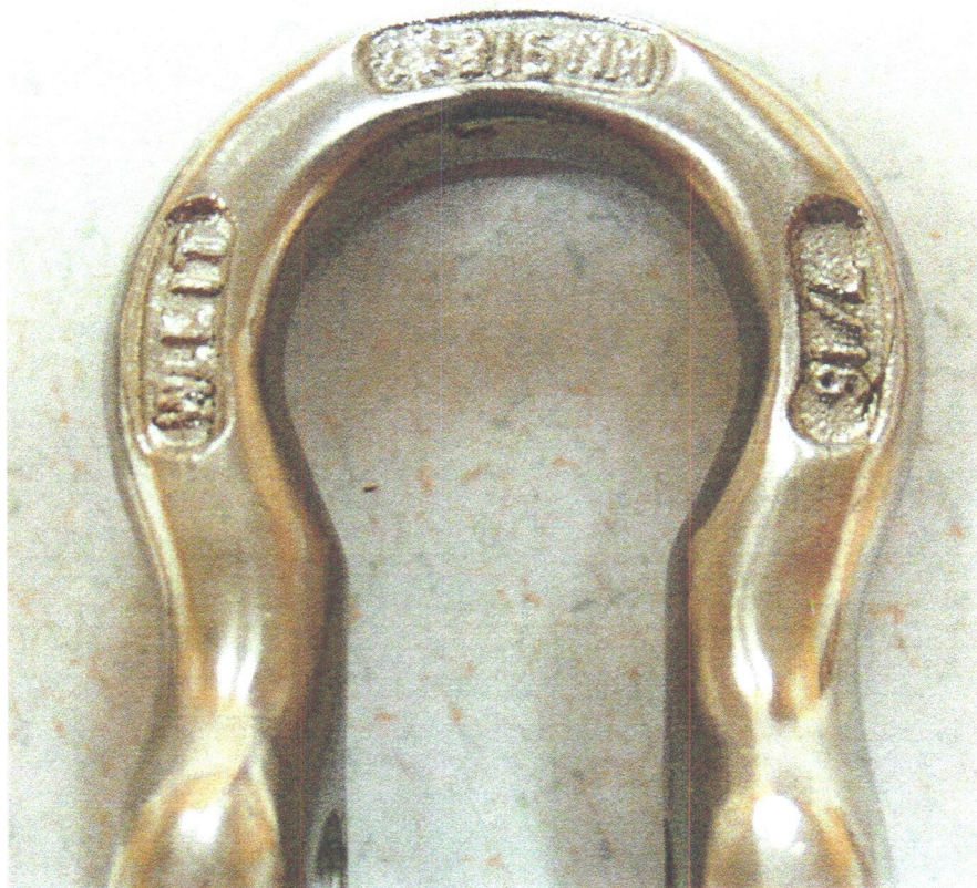
Picture # 1 Affected Anchor Shackle (BAD Shackle)
