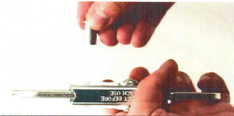
Figure 7: Fully removed rivet
