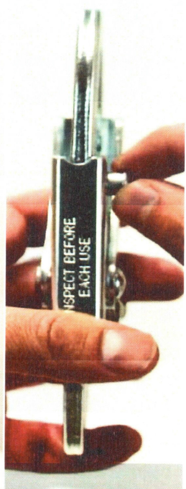
Figure 6B: Use opposite hand to pull rivet free of hook
